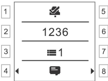
Once upon an alarm root cause is solved, the display will show . Then a reset can be performed. When confirmed and deactivated alarms , press button 7 to go to the notification reset screen. In the reset screen , press 3 or 7 to switch between notifications/ alarms and reset screens.
