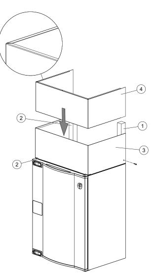
2 Fasten the upper duct cover with screws in each side.
