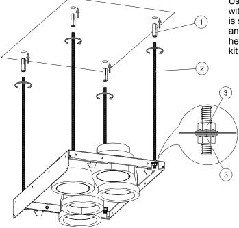
Use a 12 mm drill to make 4 holes in the ceiling with a depth of 40 mm. Distance between holes is shown in dimensions drawing. Install drop-in anchors (1) and attach threaded rods (2). Use hex flange nuts (3) to mount ceiling mounting kit on threaded rods.
