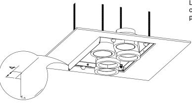
Leave at least a 4 mm gap between ceiling mounting kit and false ceiling to prevent vibration noises.
