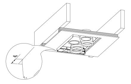
Screw battens with a ceiling mounting kit to the main ceiling. These screws are not included. Choose them based on your ceiling structure.
