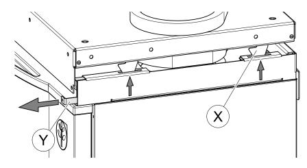
Lock hooks (X) should go through brackets. Pull out the lock mechanism (Y) if needed.
