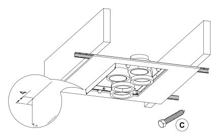
Screw anti-vibration brackets with a ceiling mounting kit to the main ceiling. Use included screws (C).
