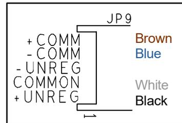
Figure 10: Sensor Wiring Color Code – Control Board
