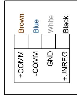
Figure 11: Sensor Wiring Color Code – Sensor Board
