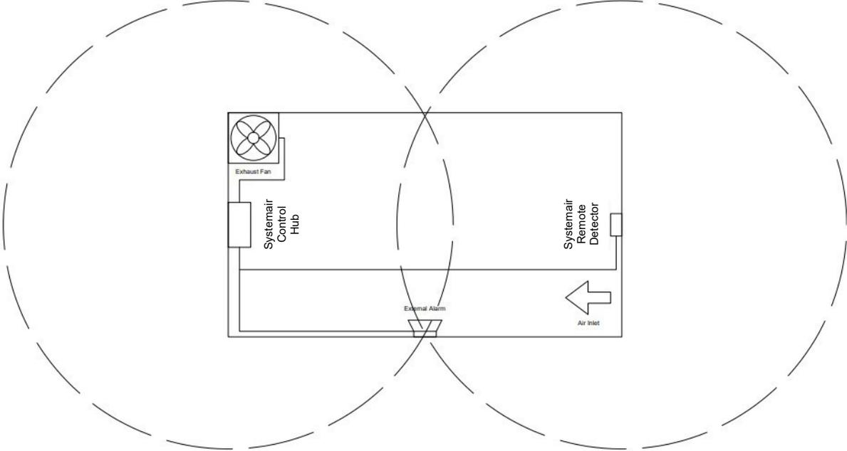
Systemair CH-S Single-Zone Control Hub Wiring – Typical Layout
