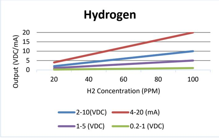
Figure 13: Proportional Output Scales (OFFSET ON)
