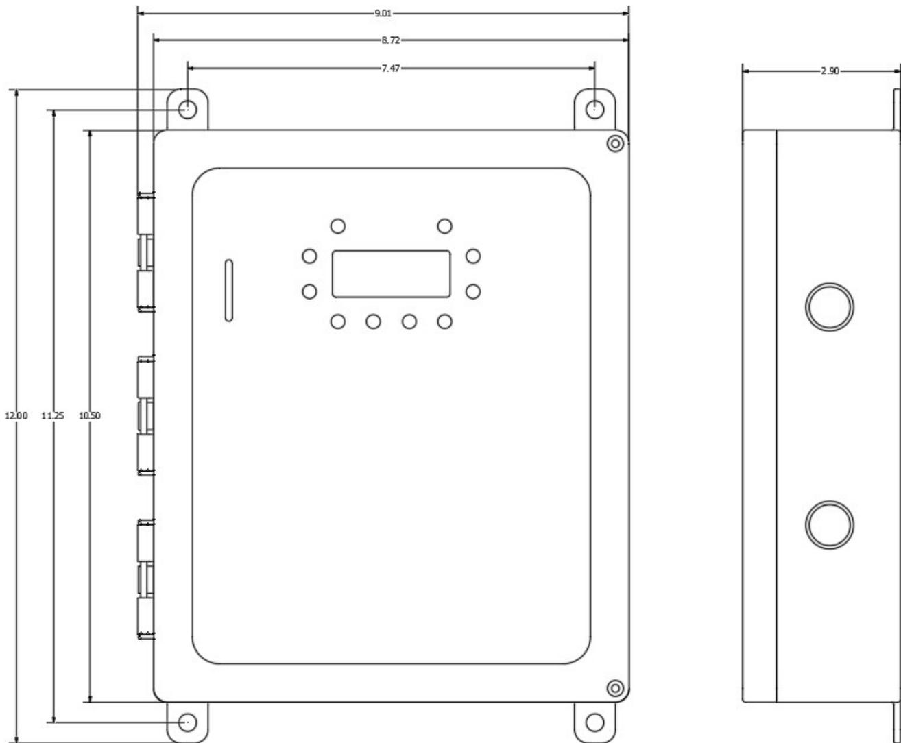
Figure 15: Dimensions (Inches – Not to Scale)
