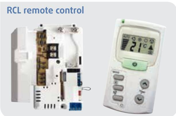
Aqu@Net controller can be provided with NIU interface card to be used with µBMS or eNIU interface card for connection to a BMS via ModBus protocol.
