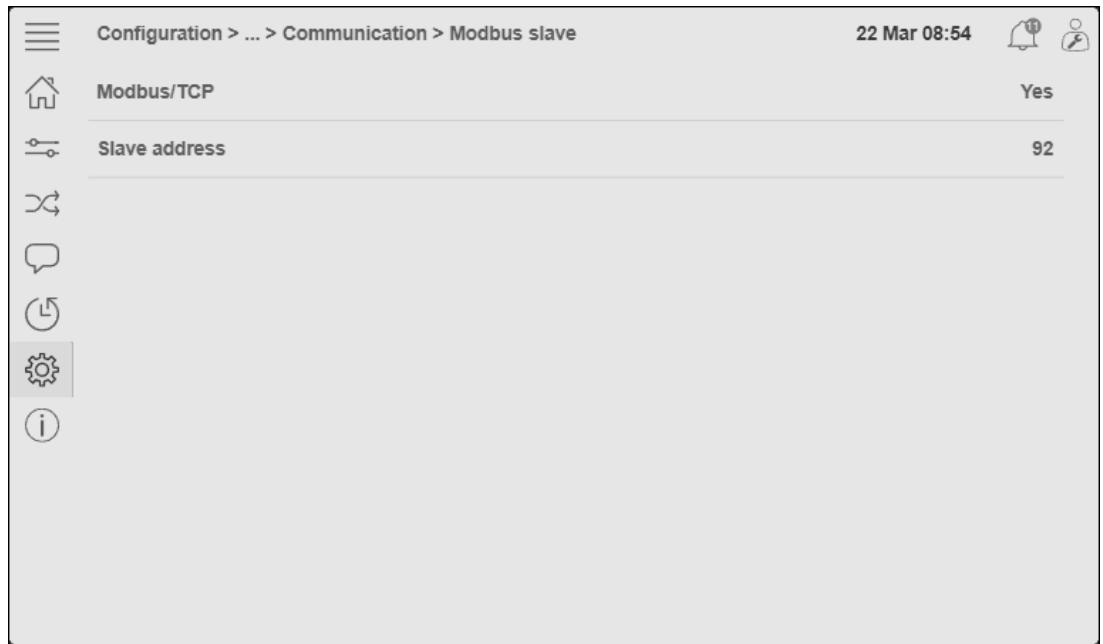
For Modbus TCP, use the controller ethernet port combined with its IP address and the TCP port 502. The port number is not changeable.
