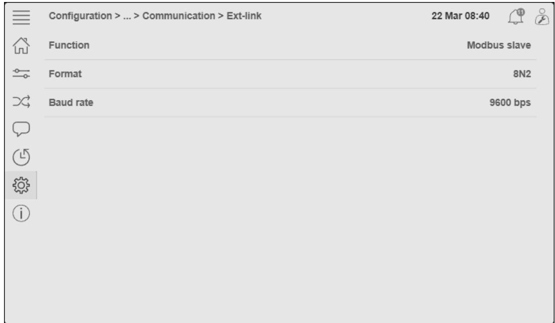
Configure the communication parameters for the Modbus-line first. The parameters defines the structure of messages and of the transmission speed. The parameters must be identical in both master and slave units.
