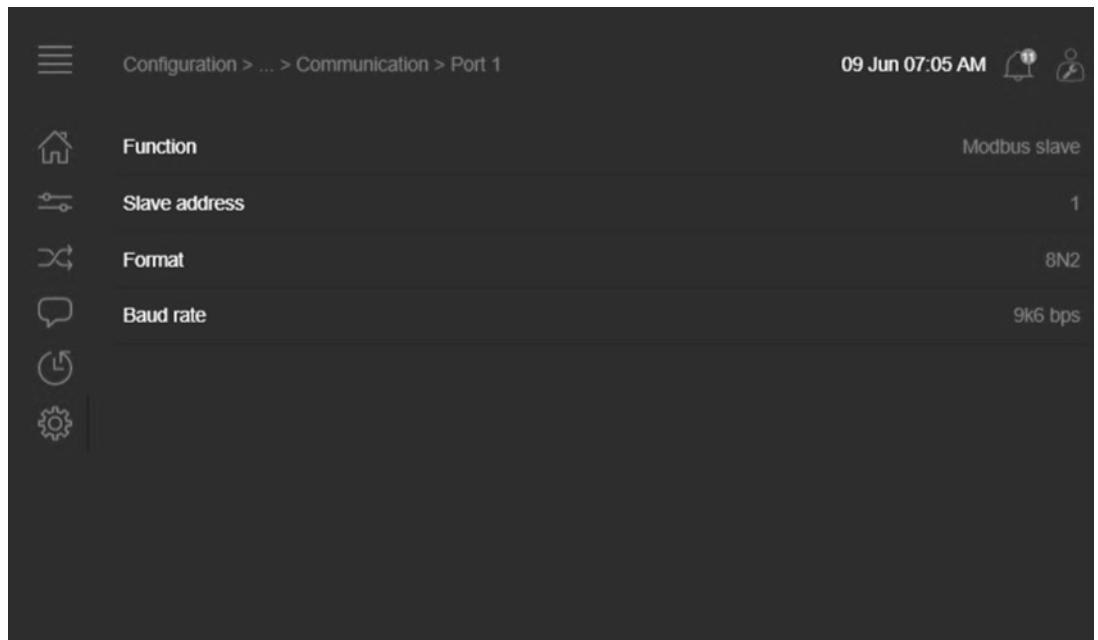
Configure the communication parameters for the Modbus-line first. The parameters define the structure of messages and of the transmission speed. The parameters must be identical in both master and slave units.
