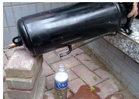
Figure 6-2.5: Draining oil from a compressor
