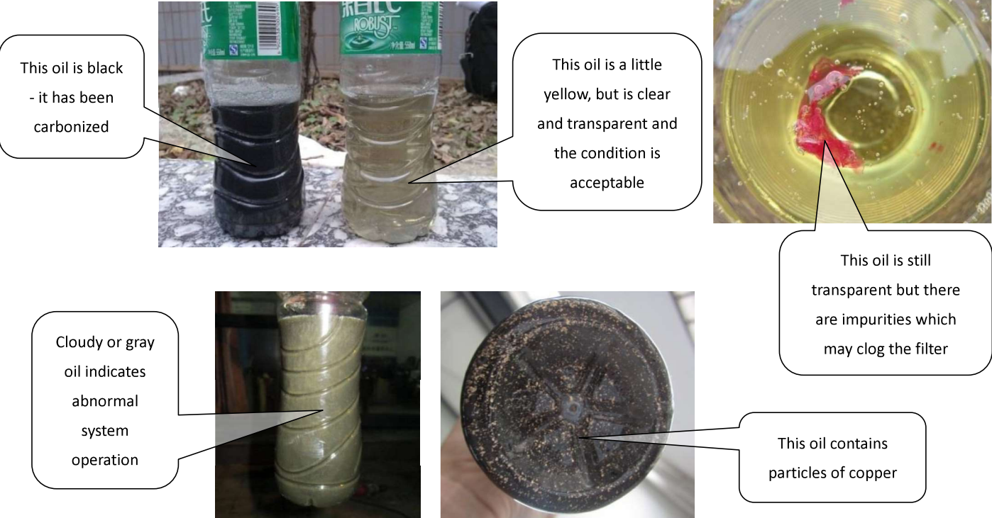
Figure 6-2.7: Inspecting compressor oil
