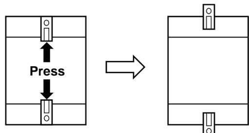
*Clips in their original position (for DIN rail mount)*      *Clips in position for wall mount*
