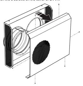
2. Attach the back plate of CVVX with 4 screws to the wall. Screws are not supplied by Systemair
