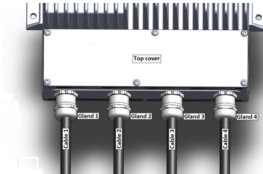
Fig.2: Description of cables
