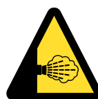
SAFETY VALVE VENTS
