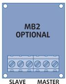
Shielded twisted single pair cable with screen 0.33 mm<sup>2</sup> to 0.5mm<sup>2</sup> (AWG 20/22)
