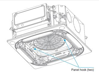
Tighten the screws under the panel hooks until the thickness of the sealing sponges 1 and 2 between the IDU and the panel outlet is reduced to about 4-6mm. The edge of the panel should be in good contact with the ceiling.
