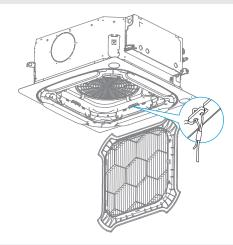
Install the suction grille back into the corresponding position, and push it up slightly at the grille clamp position to ensure that the grille buckle is fully engaged in the slot of the panel, and the grille is in the closed position.
