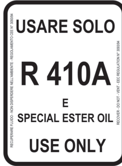
Identification of the refrigerant - External door
