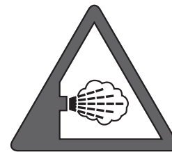
Warning - safety valves' vents
