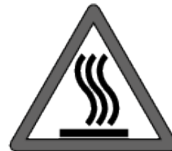
Warning - high-temperature zones Adjacent to hot pipes or components
