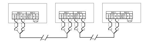
To reduce the risk of interference, the communication BUS should be terminated at each end, i.e. in the units that are located at the start and at the end of the BUS respectively. On delivery, all buses are pre-connected with a 120 Ohm resistor between terminals HI and LO on BUS2. When making further connections, remove the resistor. As an alternative to resistance, the termination switch on the board can be set to the "ON" position.
