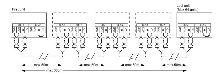
To reduce the risk of interference, the communication BUS should be terminated at each end, i.e. in the units that are located at the start and at the end of the BUS respectively. On delivery, all buses are pre-connected with a 120 Ohm resistor between terminals HI and LO on BUS2. When making further connections, remove the resistor. As an alternative to resistance, the termination switch on the board can be set to the "ON" position.
