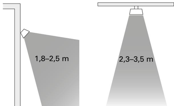
Fig.1: The heaters should heat from at least two directions for even heating
