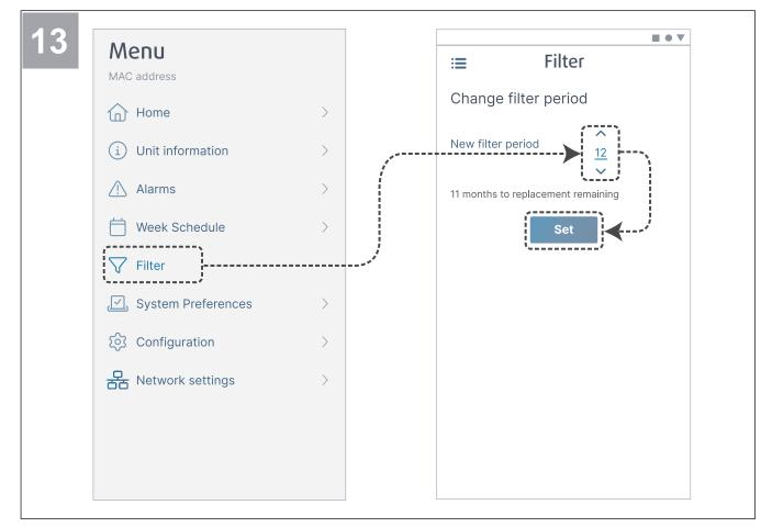
Reset filter change timer and set new filter period. Press the button **Set** to save changes.
