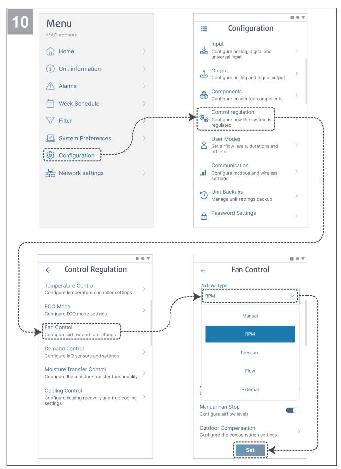
If necessary, change the type of fan control. Press the button **Set** to save changes.
