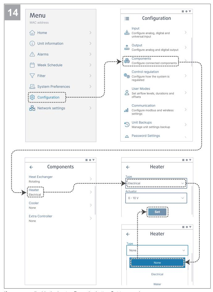
If necessary, disable the heater. Press the button **Set** to save changes.
