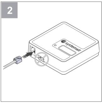
Connect the cable (B) to the SAVE CON-NECT module. Do not use USB-C port. It is for service purpose only.
