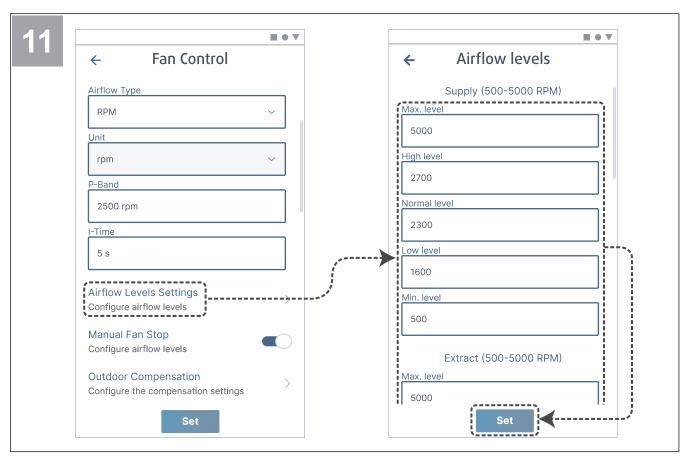
Configure supply and extract fan speed for each airflow level. Press the button **Set** to save changes.
