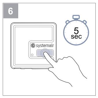
Press and hold the button for 5 seconds until the red LED starts to flash fast.
