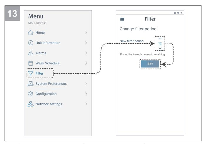
Reset filter change timer and set new filter period. Press the button **Set** to save changes.
