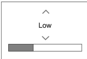
Use up and down arrows or a slider to change the airflow value.
