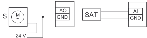
Fig. 13 Duct cooler connections
