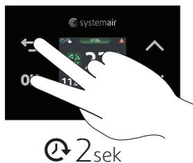
Function is activated with pressing **OK** and for 2 seconds. In status bar is showed simbol , Which mean keyboard is locked. Operation of the keys is disabled. For deactivation of function, again simultaneously press **OK** and for 2 seconds.
