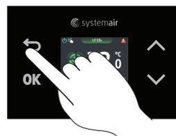
Entering of Quick menu is done with the key . Key is for selecting between Temperature view and Alarm screen. With **OK** key Home menu is available.
