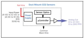
Figure 3: Wiring
