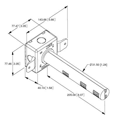
Systemair-2 CO2 duct sensor Dimensions (All Dimensions are in MM [Inch].)
