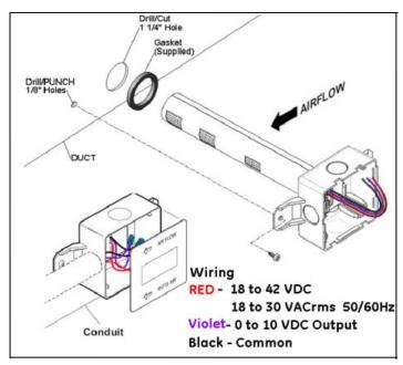
Figure 2: Systemair-2 CO2 duct sensor Installation
