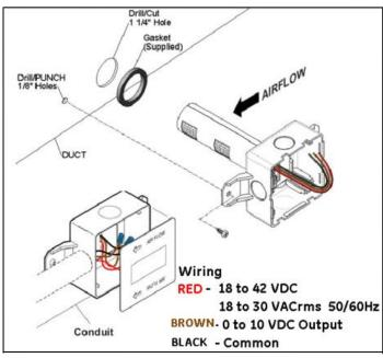
Figure 1: Systemair-1 CO2 duct sensor Installation
