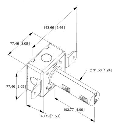
Systemair-1 CO2 duct sensor Dimensions (All Dimensions are in MM [Inch].)
