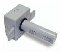
The Duct Mount CO<sub>2</sub> Sensors are transmitters designed to be installed in HVAC return air ducts. The technology is based on the absorption of light in a gold-plated reflective light pipe or waveguide diffusion gas chamber. A gas permeable PTFE filter prevents particulate and water contamination of the sensor. Light is absorbed in proportion to the CO<sub>2</sub> concentration and the
