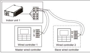
Figure 7.7 Indoor unit 1 Indoor unit 2 Indoor unit n(n<=16) क्कि कि कि D2D Wired controller 2 Master wired controller Slave wired controller
