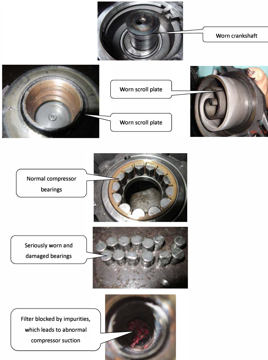
Figure 6-2.11: Effects of spoiled compressor oil
